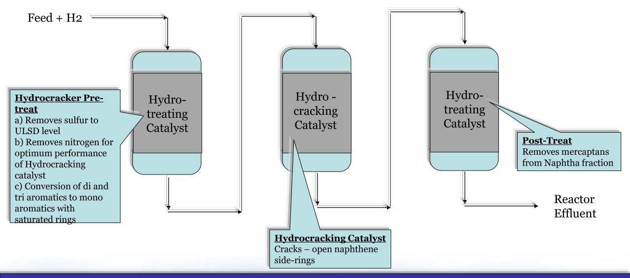
Three Processes: Pre-treatment (Hydrotreating) / Hydrocracking / Post-treatment (Hydrotreating)
